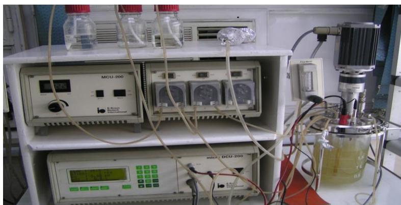
Figure 2: B-Braun Biotechnology International stirred tank bioreactor (2 L).
